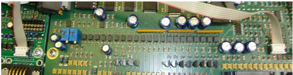
New method by using MIC-connection (same flat-cable as used for connecting to option-cards X6 / X7)
