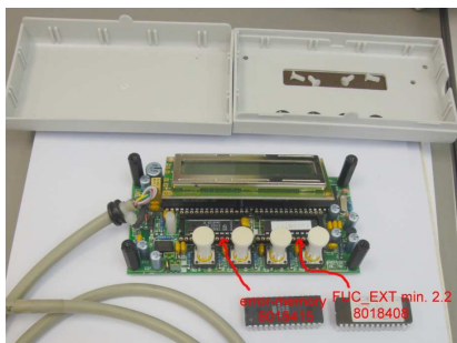
(picture shows how to place the-EEproms into the old FU-Control)
